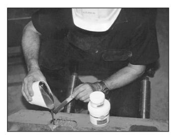
STEEL LIQUID is a pourable steel epoxy liquid that can be used in casting, filling and levelling applications. It cures to a tough inert material that may be machined, drilled or tapped later if required. The innovative technology used in the development of this product results in a finish that can also be easily applied to equipment to maximize service by providing protection against corrosion and chemical attack.
