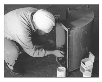
HIGH TEMP AR (Abrasion Resistant) BRUSH ON is an advanced thixotropic liquid that contains abrasion resistant ceramic particles suspended within a high performance epoxy resin. The product can be easily applied by brush to equipment to provide maximum protection against abrasion, corrosion and chemical attack whilst operating at extremely high temperatures. TYPICALLY USED ON:
