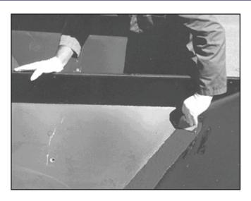
HD (Heavy Duty) CERAMIC PUTTY is a tough, impact and abrasion resistant trowellable epoxy putty specifically developed for use in extremely aggressive wear and abrasion applications. It contains highly abrasion resistant ceramic particles suspended within a high strength resilient epoxy resin.
