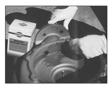
ABRASION RESISTANT PUTTY is a fine grade trowellable abrasion resistant epoxy developed for smooth, low friction treatment and repair of equipment. It contains a blend of specially graded ceramic particles to provide maximum resistance to abrasion in high wear applications.
