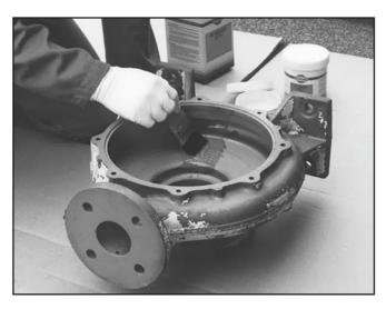
CERAMIC BRUSH ON is a highly advanced thixotropic liquid that contains highly abrasion resistant ceramic particles suspended within a high strength epoxy resin. This coating can be easily applied by brush to equipment to maximize service life by providing protection against abrasion, corrosion and chemical attack. Available as Red, Blue or White.
